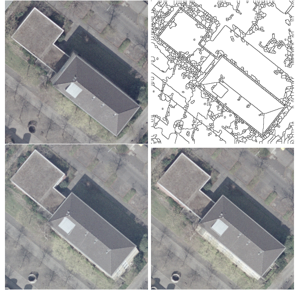
Figure 1: Three aerial views of a building scene consisting of a flat roofed part and a gable roofed part. The initial segmentation of the upper view is shown on its right side. The ground consists of several weirdly shaped regions, and the flat roof is also not well segmented.
