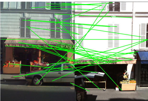
Figure 3: SIFT points matching between a query taken with a mobile phone and an image from the iTowns database.
