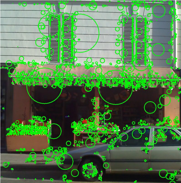
Figure 2: SIFT points of interest with respecting scales.
