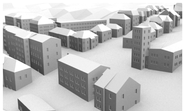
Figure 10. Facade geometry synthesized from grammar library
