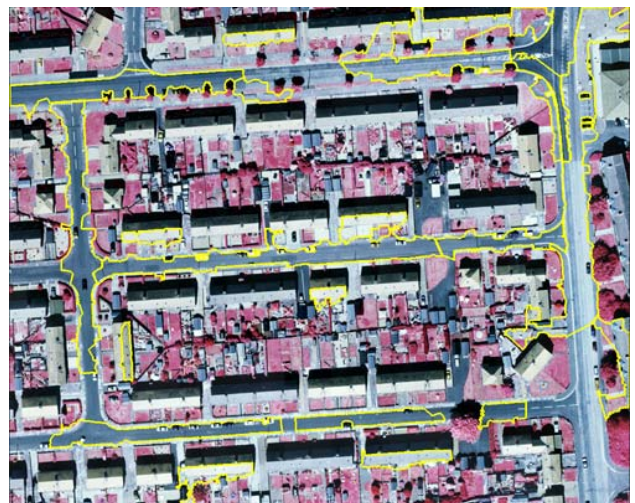
Figure 3. Road parts extracted in subset 1 (yellow).
