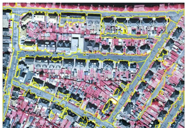
Figure 4. Road parts extracted in subset 2 (yellow).
